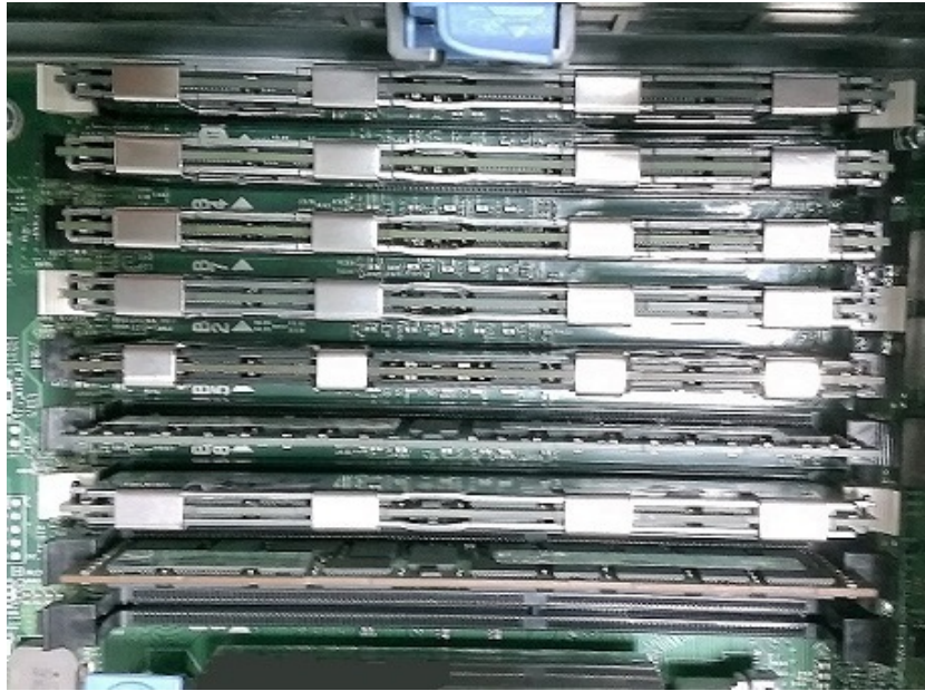
Figure 9.2. ECC RAM modules placed in memory banks
