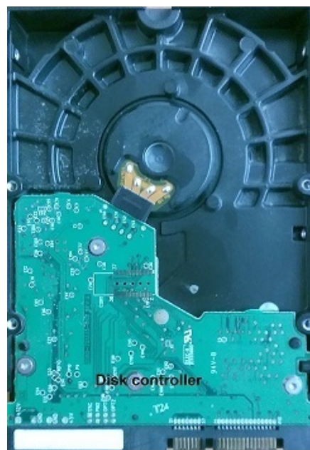
Figure 8.5. Disk controller in HDD
